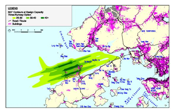
Figure 5.51 : Preliminary Projection of Three-Runway NEF Contours for HKIA at Design Capacity
