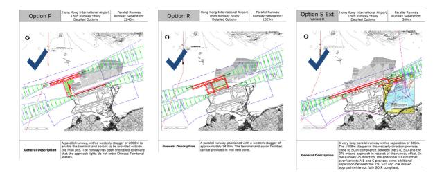
**5.8** The 15 alignment options can indeed be categorised into three main families of alignment options for evaluation in terms of operational safety, obstacle clearance, PRD airspace constraint issues, air traffic control procedures, and optimum mode of operations including runway usability and capacity.
