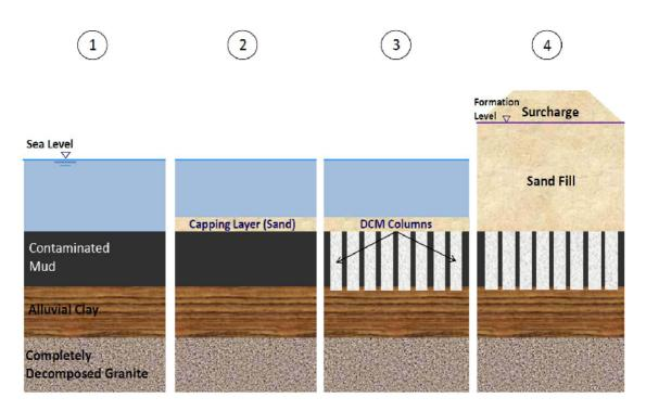
**5.65** Sand fill compacted by vibro-compaction is proposed as the key fill material for the reclamation. In all areas, surcharge preloading is proposed to control the anticipated settlement during the service life of the landfill. The duration of surcharge preloading will depend on the results of instrumentation monitoring throughout construction but is anticipated to be in the range of 4 to 12 months.
