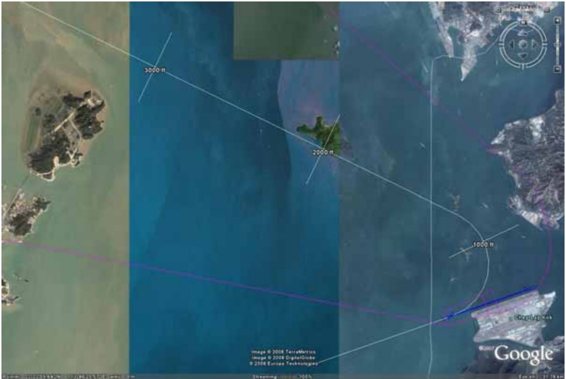
Figure 5.22 Option S Extended (Variants A, B and C) Runway 07L 135 degree Missed Approach 185 knots
