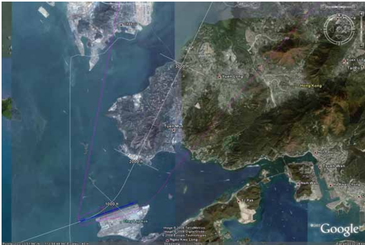
Figure 5.21 Option S Extended (Variants A, B and C) Runway 07L 45 degree Missed Approach
