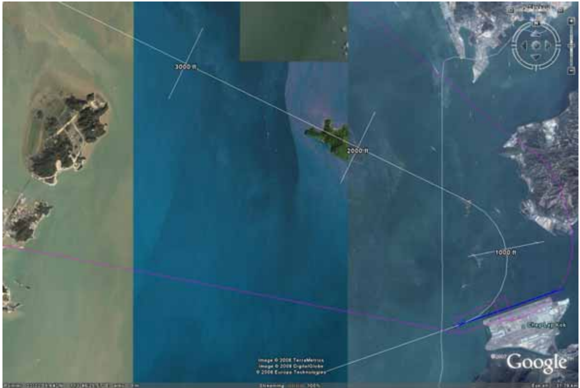
Figure 5.31 Option S Extended (Variants D and E) Runway 07L 135 degree Missed Approach 200 knots
