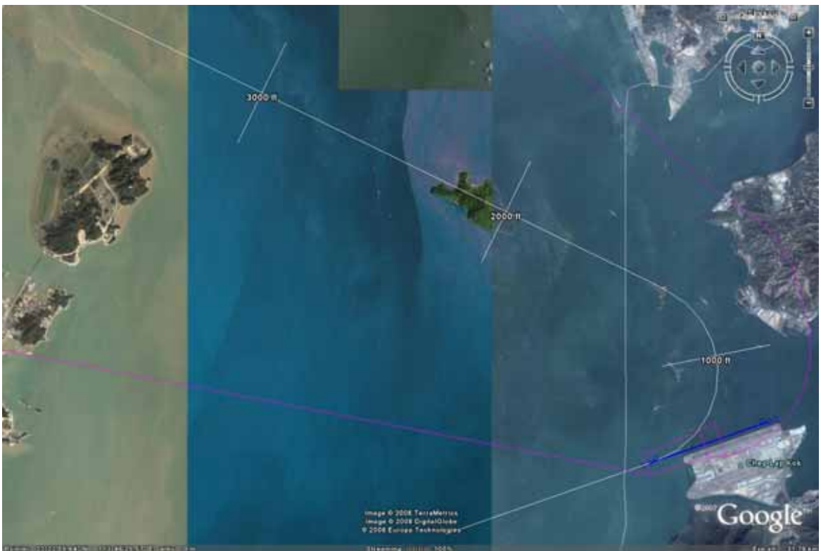
Figure 5.23 Option S Extended (Variants A, B and C) Runway 07L 135 degree Missed Approach 200 knots
